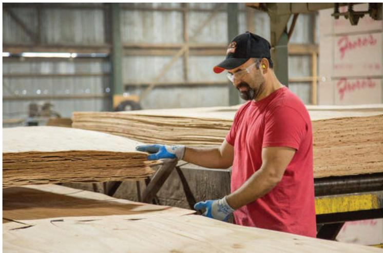
**Plywood manufacturing at a Freres Lumber Company facility.**
